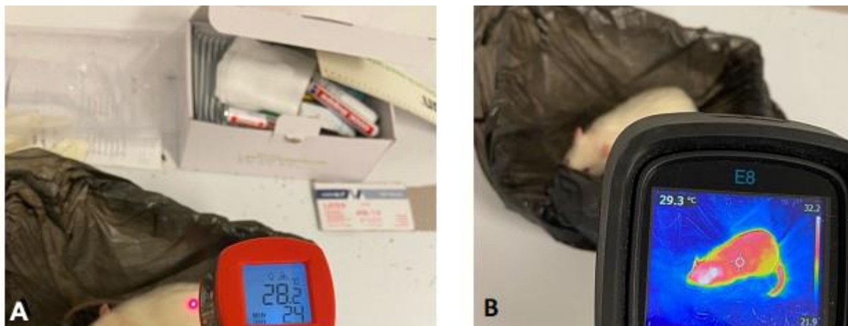
Fig. 2: Temperature measurement on the animal's back using infrared A) IRT and B) TIC.
