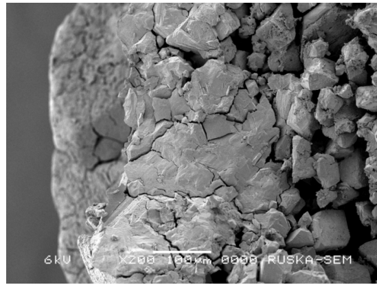
Fig. 5: Scanning electron micrograph showing large sized magnesium ammonium phosphate crystals even towards the periphery.
